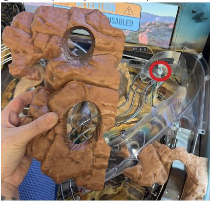
Remove the old clear plastic to be replaced by the newly shaped clear plastic:
