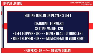
Figure 3-15. Topper Test/Adjust - edit servo limits.
