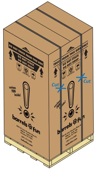
Figure 1-2. Removing straps from the shipping carton/pallet.
