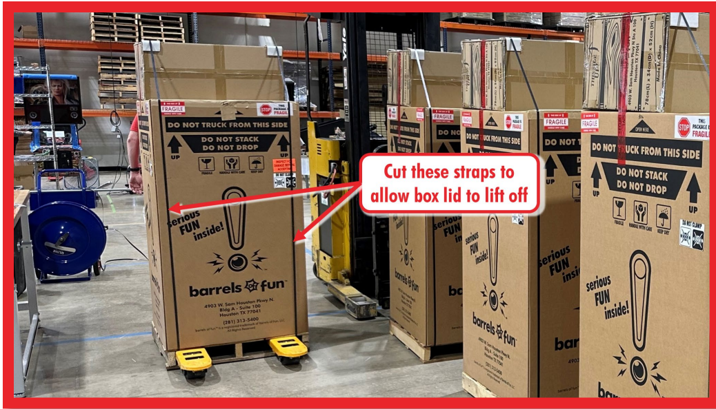
DOMESTIC – LARGER BOX LID SECURED WITH STRAPS
