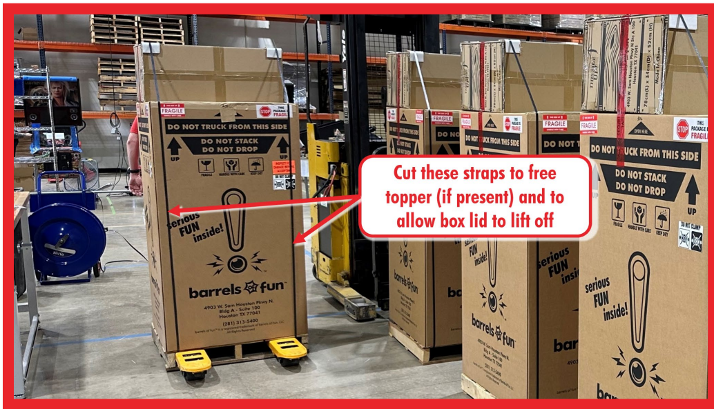
DOMESTIC – LARGER BOX LID SECURED WITH STRAPS
